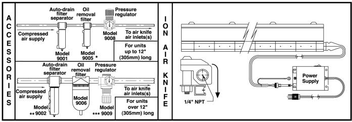
\* Use Model 9006 Oil Removal Filter for Ion Air Knives longer than 6" (152mm)
