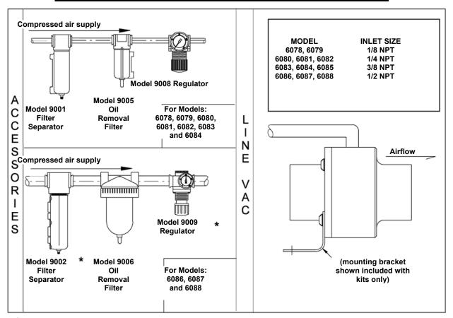
For Model 6085 - Use Model 9032 Filter Separator and Model 9033 Pressure Regulator
