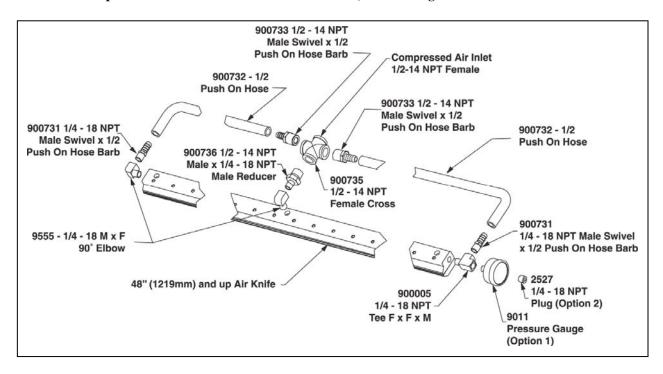
Pipe thread sealant should be applied to all threads (small packet included). Avoid the inside diameter of the fitting so it does not enter into the Air Knife.
