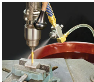
A Model SR1010SS is used to supply a cooling mist for a drilling operation.
