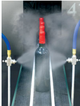
(2) Model EB1040SS nozzles are used to rinse wine bottles after capping.
