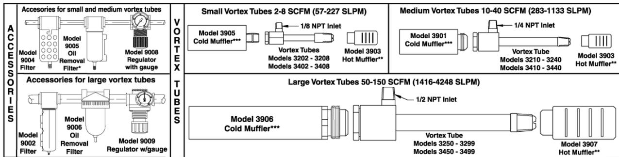
\*Use Model 9006 Oil Removal Filter for Vortex Tubes larger than 30 SCFM (860 SLPM)
