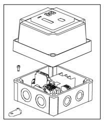
7. Position the thermocouple inside the enclosure where desired. It is not sensitive to mounting position. The thermocouple must be mounted inside the enclosure. It should not be mounted directly in the cold airstream that exhausts from the Cold Air Distribution Kit. Do not kink the wires. Ordinary tape can be used to hold the thermocouple in position.
