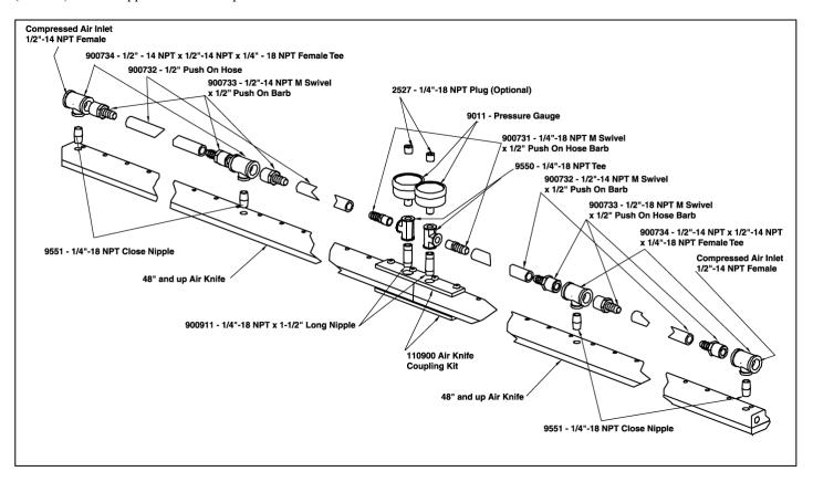
Pipe thread sealant should be applied to all threads (small packet included). Avoid the inside diameter of the fitting so it does not enter into the Air Knife.
