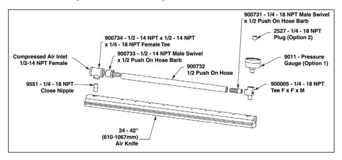
Pipe thread sealant should be applied to all threads (small packet included). Avoid the inside diameter of the fitting so it does not enter into the Air Knife.
