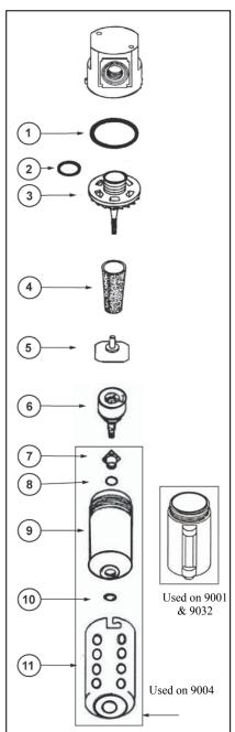
Wash filter element at intervals with naphtha to maintain filtering efficiency. To clean element, depressurize system, unscrew bowl, and unscrew element from head. Dry the filter element thoroughly before reassembling. Clean filter bowl(s) only with soapy water. Inspect O-ring, replacing if damaged or distorted. Reassemble with care to avoid stripping threads on bowl.
